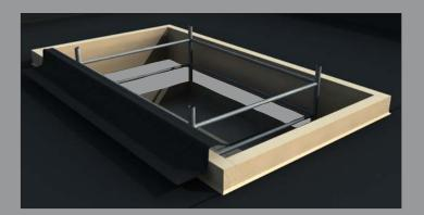
A timber kerb of 150mm high x 70mm wide (not supplied) must be fitted around the opening in the flat roof – the weatherproofing membrane laps onto the top face of the kerb.
